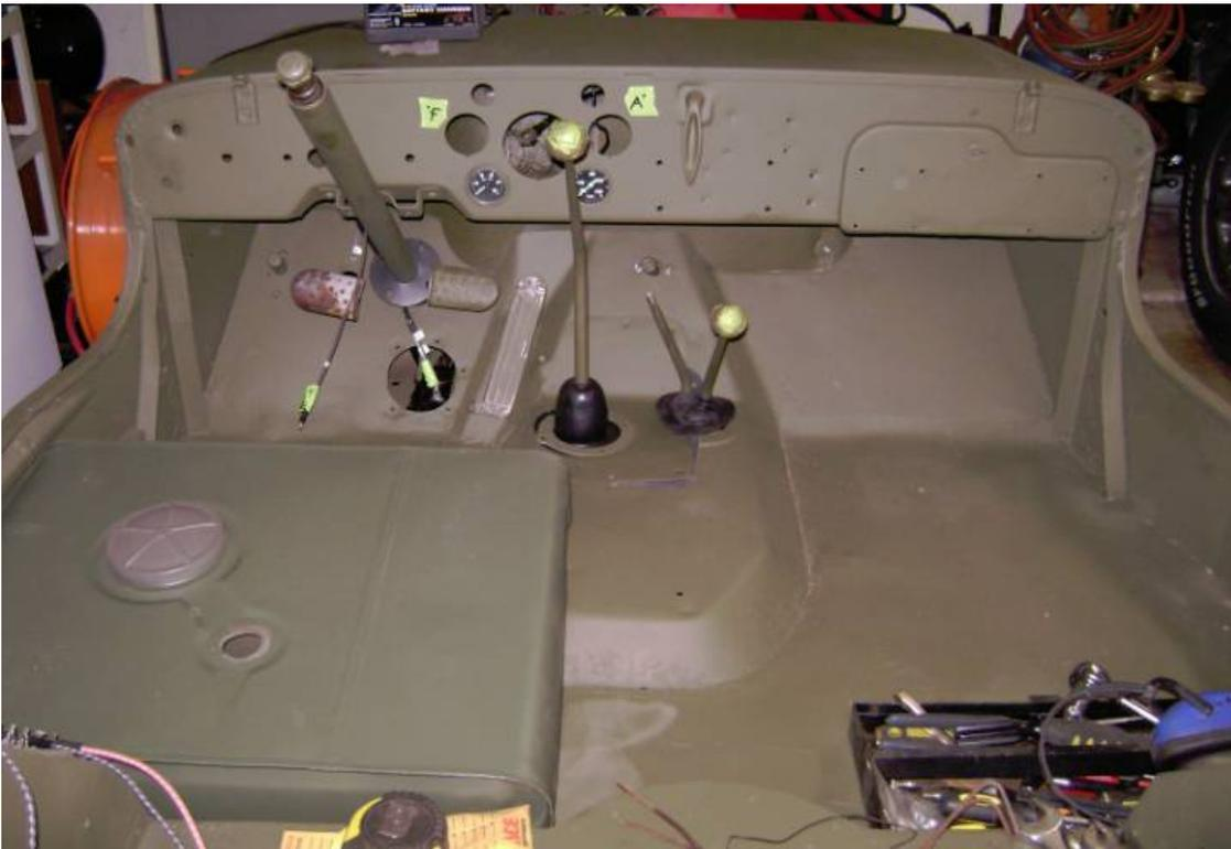
After a day of adding things. The green tape with F and A are for Fuel gauge and Ammeter. The O and T are missing as the Oil pressure gauge and Temp gauge are in place. New gas tank look great ... Laurie helped a bunch ... she place all the felt padding etc.
