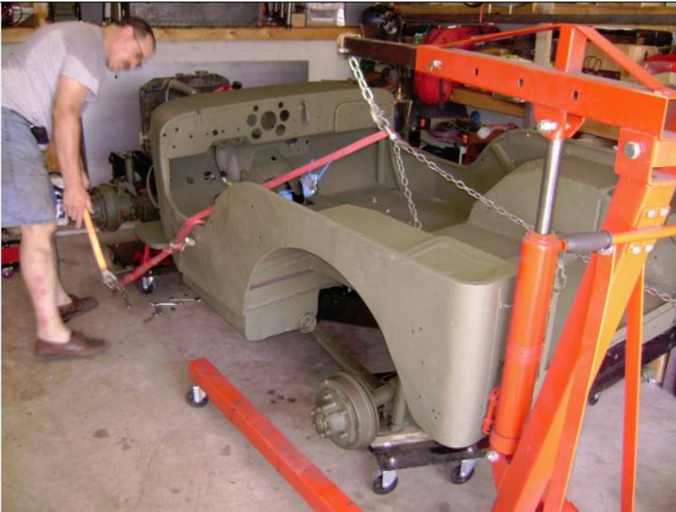
The engine lift was a God send. We could have balanced things better, but it took less time to get the body in place, than it did to get the lift hooked up. I supervised (yelled and hollered) and Jonathan pushed and tugged on the lift.
