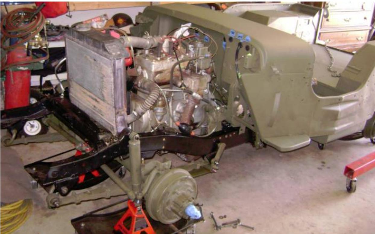
Body in place. The blue tape on the fire wall marks [all](#) the wires and cables etc. New rubber grommets are in place. The new Main wiring harness is fed into through the fire wall.
