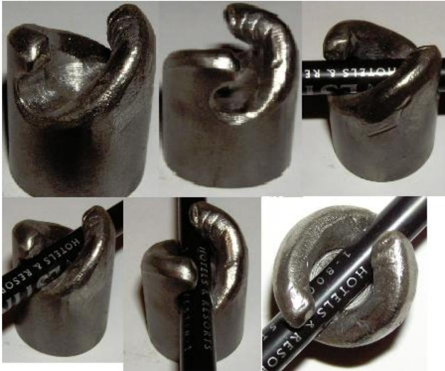
View of the finished hand crank head.
